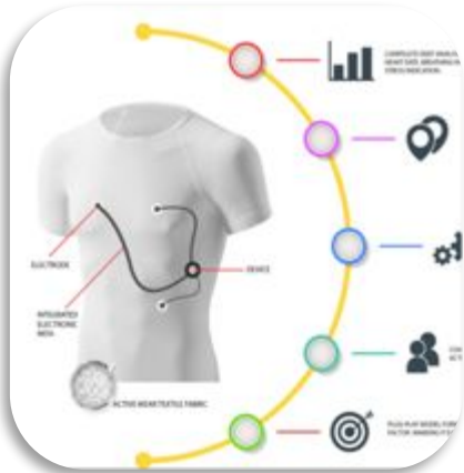
NYOKAS: Smart textile to monitor vital parameters of wearer
