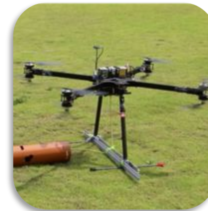
AI DRONE: Heavy lift drone capable of payloads up to 100 kgs
